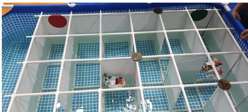
Fig. 1. Example of a possible configuration of the polygon. The width of the labyrinth corridor is 30 cm.
